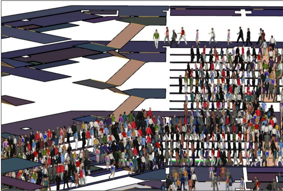
Figure 4.26. 1<sup>st</sup> elbow point (queueing on the spectator seats corridor)
