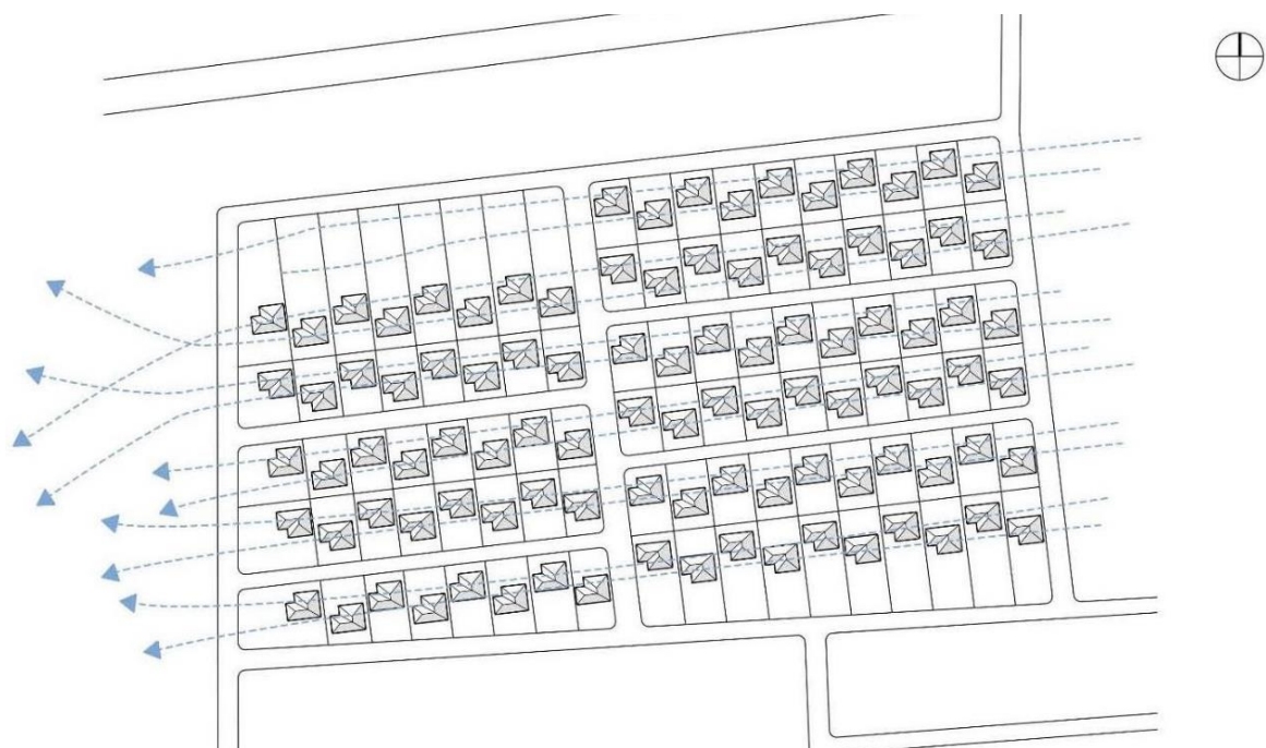
Figure 3.89. The arrangement of the 100 Houses, the graph shows the cross ventilation through houses (The Vann Molyvann project, 2015)
