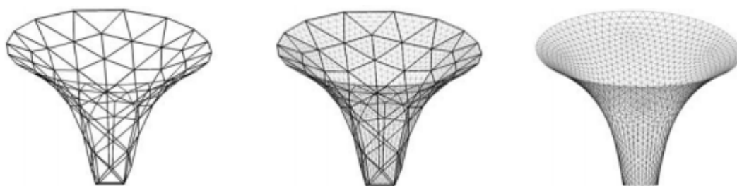
Figure 2.1. The design process of the EXPO Shanghai sun valleys, from large triangles (Left) their division (Middle) to relaxation of the grid (Right) [53]
