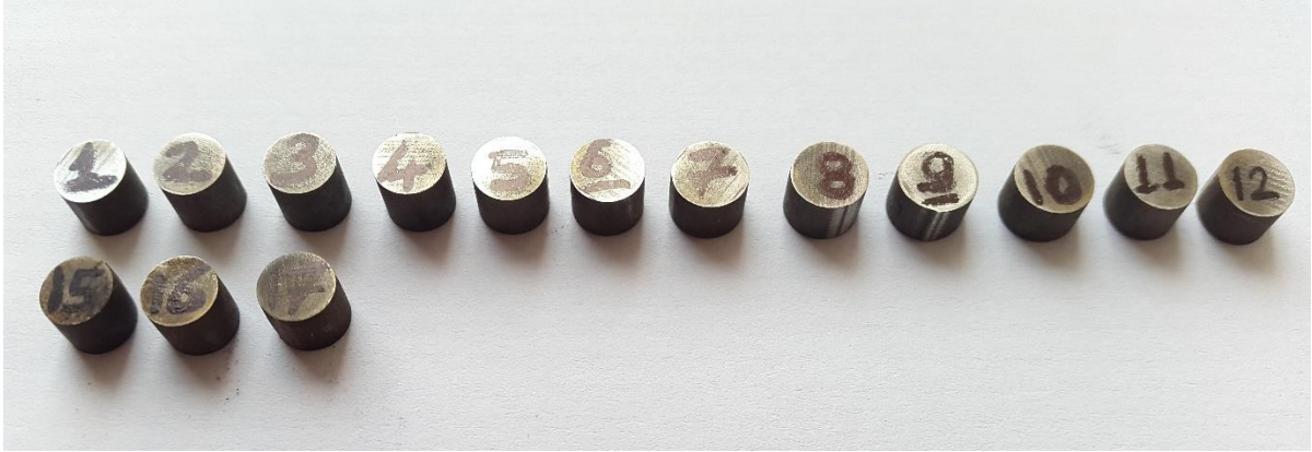
Figure 3.19. Pictures of tested cylindrical specimens in dynamic compression tests
