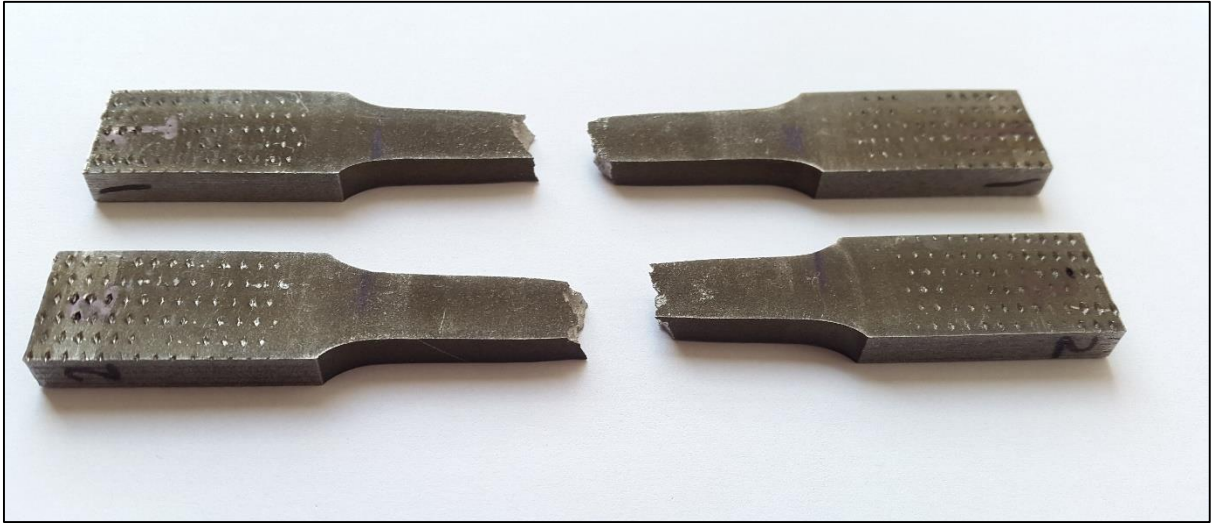
Figure 3.14. Pictures of tested tensile test specimens
