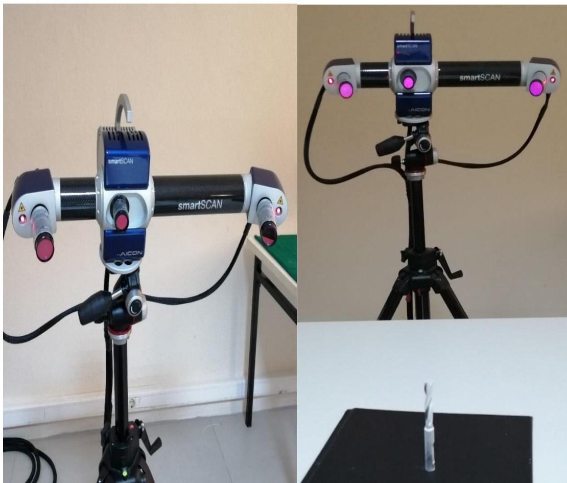
Figure 3.4. AICON Smart Scan 3D system during scanning process
