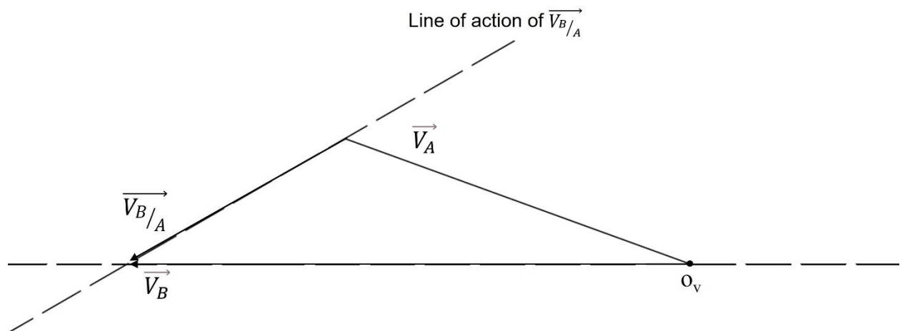
As a result of the measurements,  $\vec{V}_B$  is found to be -110 mm/s and  $\vec{V}_{B/A}$  is 39 mm/s. So the angular velocity of link 3:
