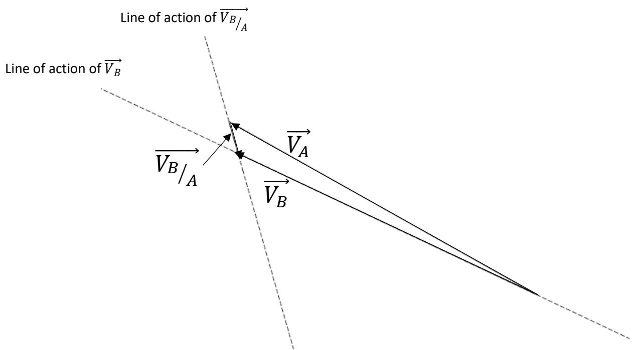
As a result of the measurements,  $\overrightarrow{V_B}$  is found to be 18.6 mm/s and  $\overrightarrow{V_{B/A}}$  is 1.44 mm/s. So the angular velocities:
