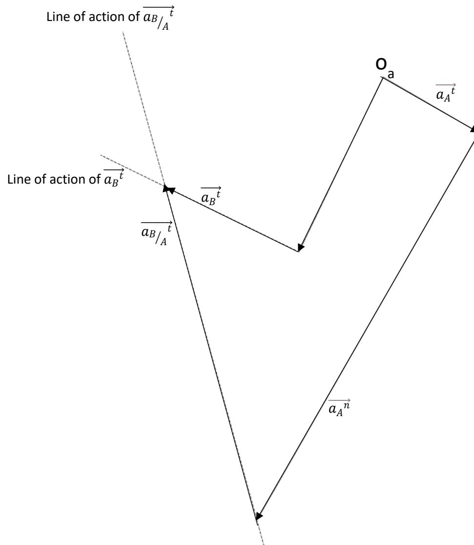
Since  $\overrightarrow{a_{B/A}^n}$  is very small compared to other accelerations, it is not seen on the polygon. As a result of the measurements,  $\overrightarrow{a_B^t}$  is found to be  $13.42 \text{ mm/s}^2$  and  $\overrightarrow{a_{B/A}^t}$  is  $31 \text{ mm/s}^2$ . So the angular accelerations:
