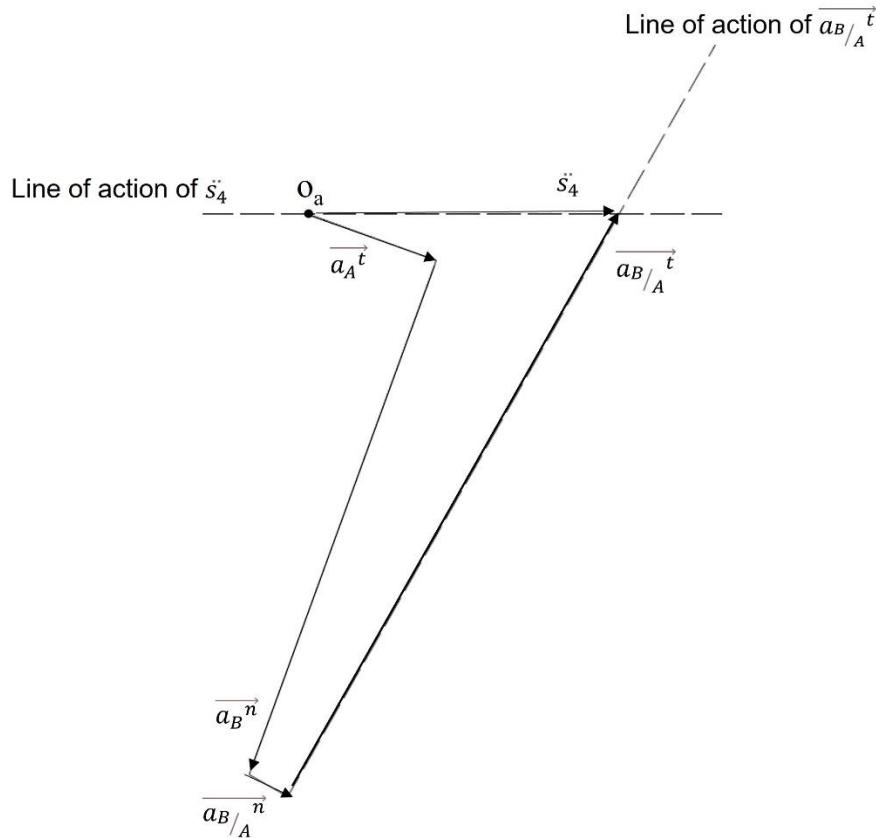
As a result of the measurements,  $\ddot{s}_4$  is found to be  $75 \text{ mm/s}^2$  and  $\overline{a_{B/A}}^t$  is  $225 \text{ mm/s}^2$ . So the angular acceleration:
