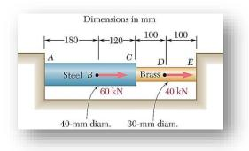
The A-36 steel bar shown in Fig.(a) is constrained to just fit between two fixed supports when  $T_1 = 30^{\circ}$ C. If the temperature is raised to  $T_2 = 60^{\circ}$ C, determine the average normal thermal stress developed in the bar.
