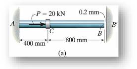
Two cylindrical rods, one of steel and the other of brass, are joined at *C* and restrained by rigid supports at *A* and *E*. For the loading shown and knowing that  $E_{st} = 200$  GPa and  $E_{br} = 105$  GPa, determine (*a*) the reactions at *A* and *E*, (*b*) the deflection of point *C*.
