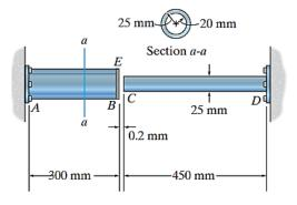
The center rod *CD* of the assembly is heated from  $T_1 = 30^{\circ}$ C to  $T_2 = 180^{\circ}$ C using electrical resistance heating. At the lower temperature  $T_1$  the gap between C and the rigid bar is 0.7 mm. Determine the force in rods *AB* and *EF* caused by the increase in temperature. Rods *AB* and *EF* are made of steel, and each has cross-sectional area of 125 mm<sup>2</sup>. *CD* is made of aluminum, and has cross-sectional area of 375 mm<sup>2</sup>.
