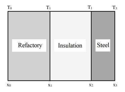
Figure. Layers in a composite furnace wall.
