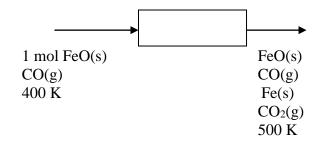
If the mole ratio of FeO(s) to CO(g) in feed is 1/0.8, calculate the heat duty Q(kJ) when fractional conversion of FeO (s) is 0.5. C<sub>p</sub> (kJ/mol.K) in terms of T(K) adapted from Perry's Chemical Engineeers' Handbook
