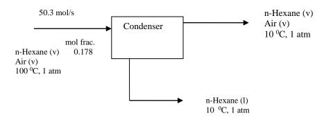
A mixture of n-Hexane and Air is fed to a condenser at a rate of 50.3 mol/s at 100  $^{0}$ C and 1 atm. The mole fraction of hexane in this mixture is 0.178. In the condenser gas mixture is cooled at constant pressure and 60% of the hexane condensed. The exit temperature of both condensed liquid and vapor side is 10  $^{0}$ C. Calculate; (a) the molar flow rates of two exit streams (b) the required cooling rate in kW. Note: When necessary, C<sub>p</sub> will be taken as C<sub>p</sub> = a + b T.
